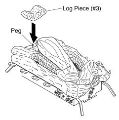
Figure 20 - Installing Log Piece (#3)
